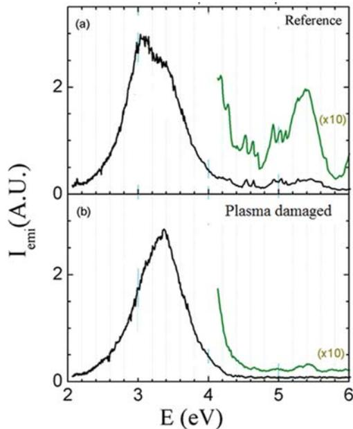
FIG. 5. (Color online) Comparison of 10 K photoluminescence spectra of (a) a reference  $\text{Ga}_2\text{O}_3$  sample and (b) a plasma damaged  $\text{Ga}_2\text{O}_3$  sample. The higher energy peaks exhibit the spectra measured in the higher sensitivity range and are enlarged for clarity.
