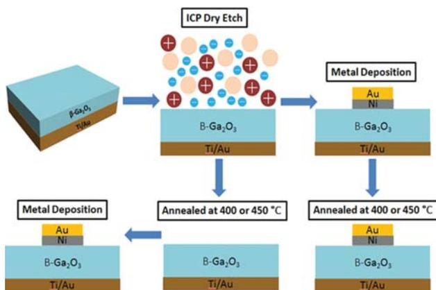
FIG. 1. (Color online) Schematic of experiment-Ni/Au Schottky diodes formed on dry etched  $\beta$ -Ga<sub>2</sub>O<sub>3</sub> surfaces either before or after subsequent annealing at 400 or 450 °C.
