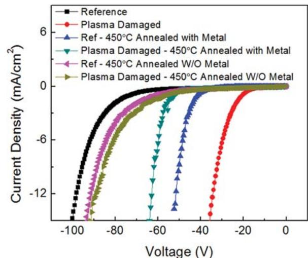
FIG. 4. (Color online) Reverse I–V characteristics of Ni/Au  $\text{Ga}_2\text{O}_3$  diodes on surfaces dry etched in  $\text{BCl}_3/\text{Ar}$  ICP discharges and annealed at 450 °C either before or after deposition of Ni/Au.
